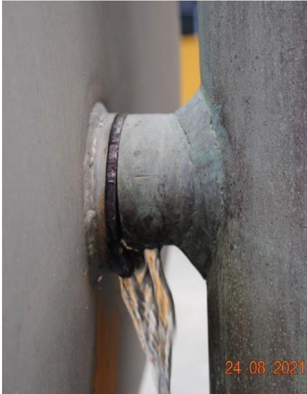
Drop & leak on larger 'bucket' Cause as for smaller buckets
