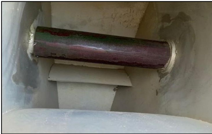
Cylindrical 'Tufnol' hopper sleeve through centre of smaller hopper/bucket
